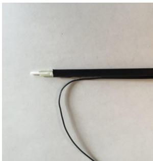
Detach tracer/toner wire & remove outer jacket and aramid fibers to desired length of fiber to be exposed. Cut strength members to 1/2" (13mm) from outer jacket. Repeat on all ends to be spliced.
