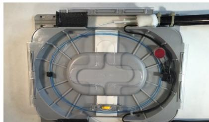
Properly assembled FOD-40 kit ready for encapsulation with splices held securely on the pressure sensitive pad.
