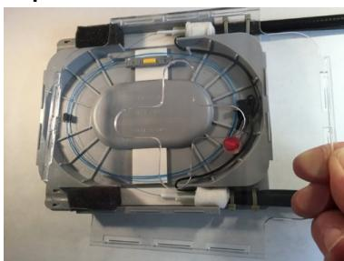
Ensure that all fibers are relaxed and laying flat in the race track between all posts and fences. Press the cover onto the base; pressing firmly until the cover engages with an audible snap. Place on a flat, level surface for filling.
