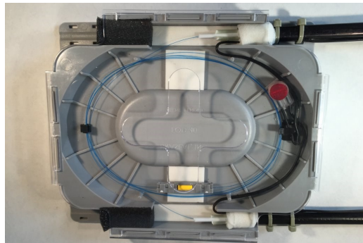
Properly assembled FOD-40 kit ready for encapsulation with splices held securely on the pressure sensitive pad.
